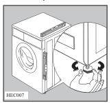
Any necessary adjustment can be made with a spanner. Accurate levelling prevents vibration, noise and displacement of the machine during operation. Some vibration is inevitable, especially if mounted on a
